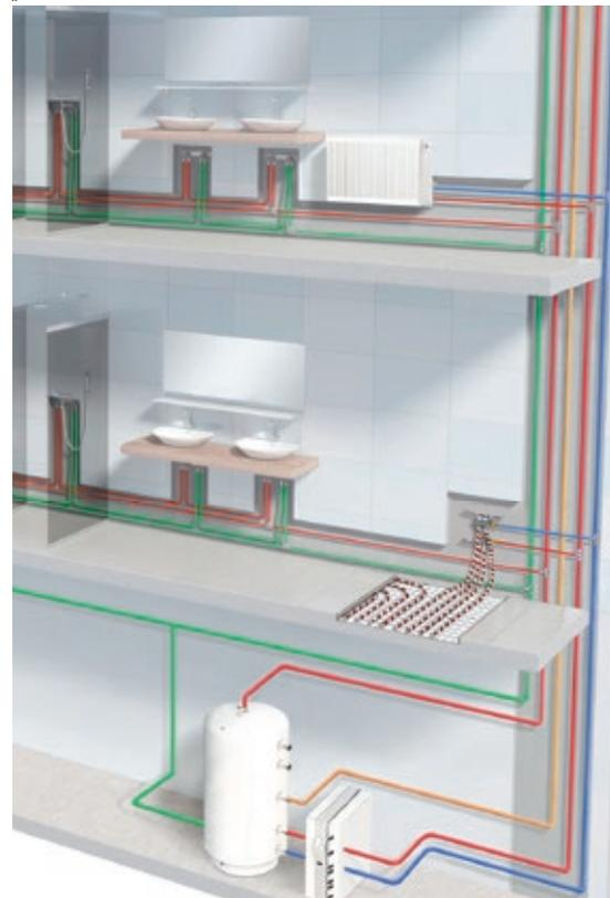
**58 % energy saving with 2-pipe systems compared to central domestic hot water systems\***
